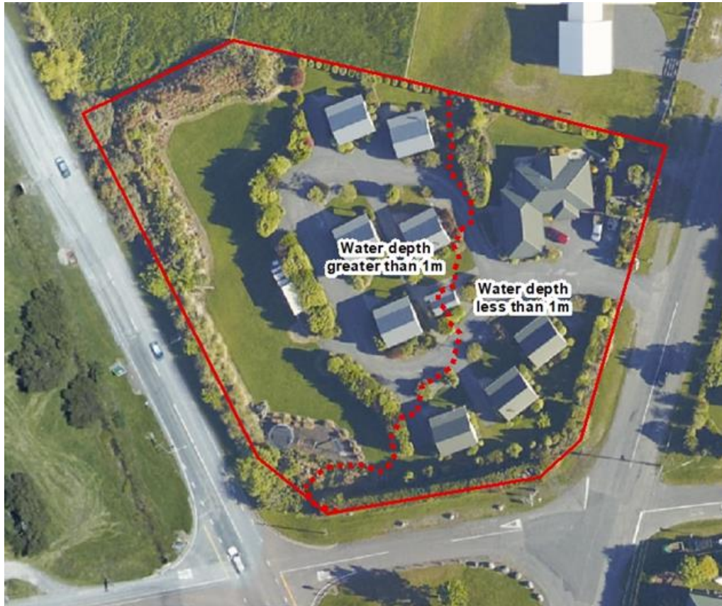
Image above shows the 'Indicative 500 year maximum ARI water depth for 7 Old Beach Road'. Note – ARI = Average Recurrence Interval (provided by ECan)
