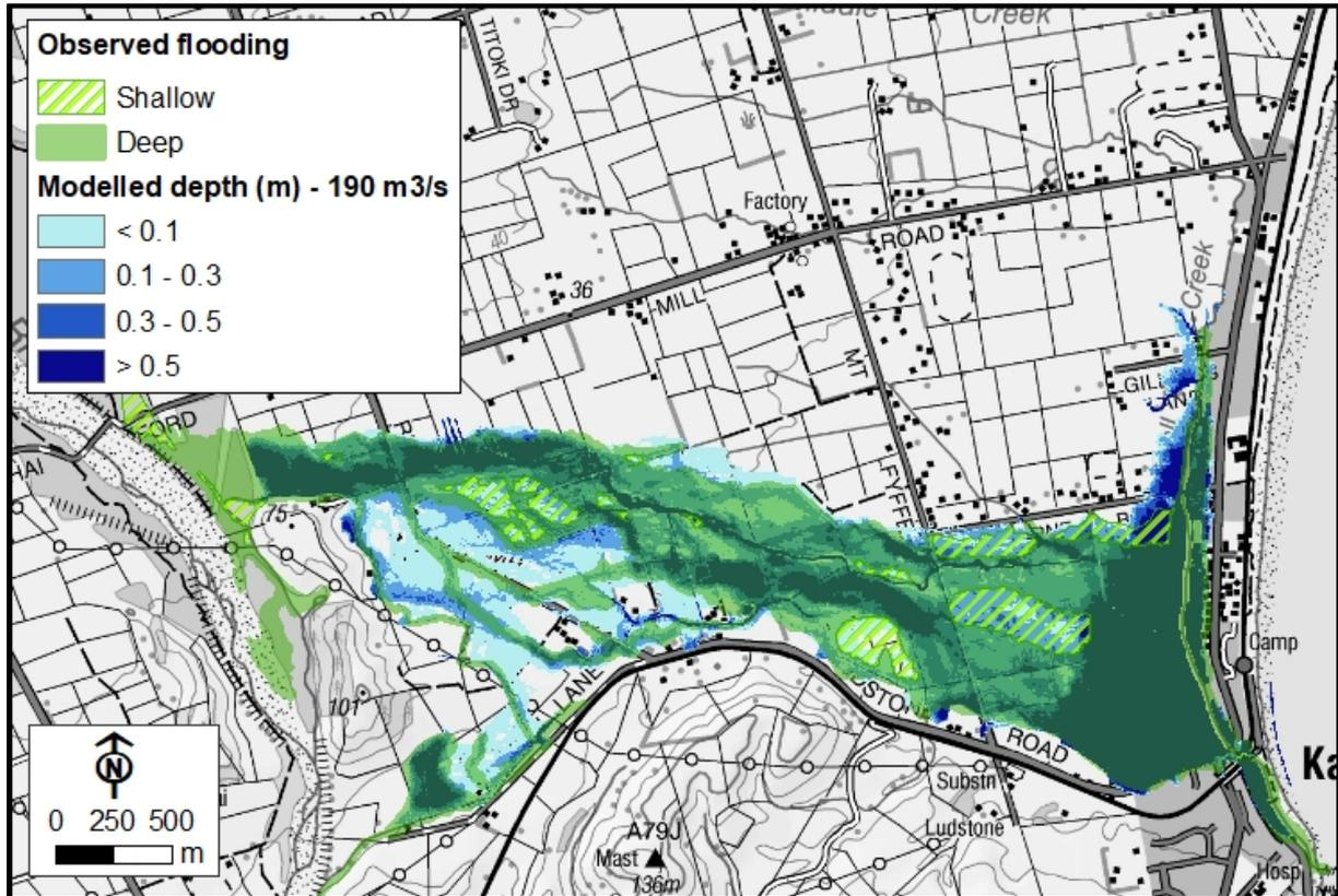
Figure 3-10: Comparison of observed and modelled flooding for the December 1993 flood event with a Kowhai River breakout of 190 m<sup>3</sup>/s
