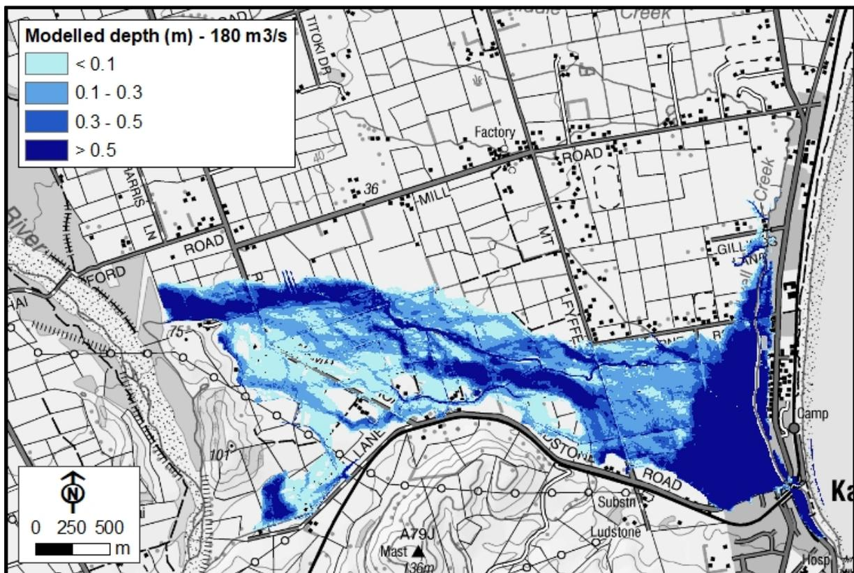
Figure 3-11: Modelled flood depths for the December 1993 flood event (Breakout of 180 m<sup>3</sup>/s)
