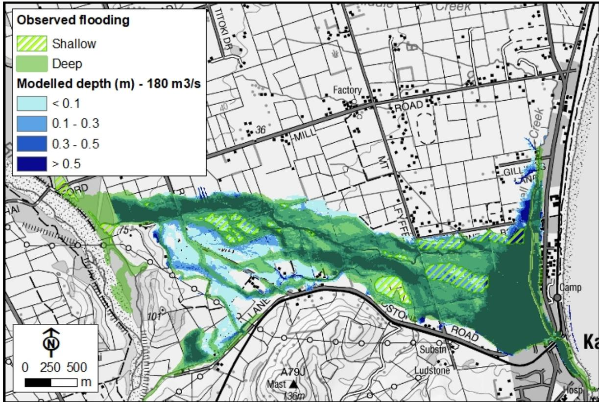
Figure 3-12: Comparison of observed and modelled flooding for the December 1993 flood event with a Kowhai River breakout of 180 m<sup>3</sup>/s
