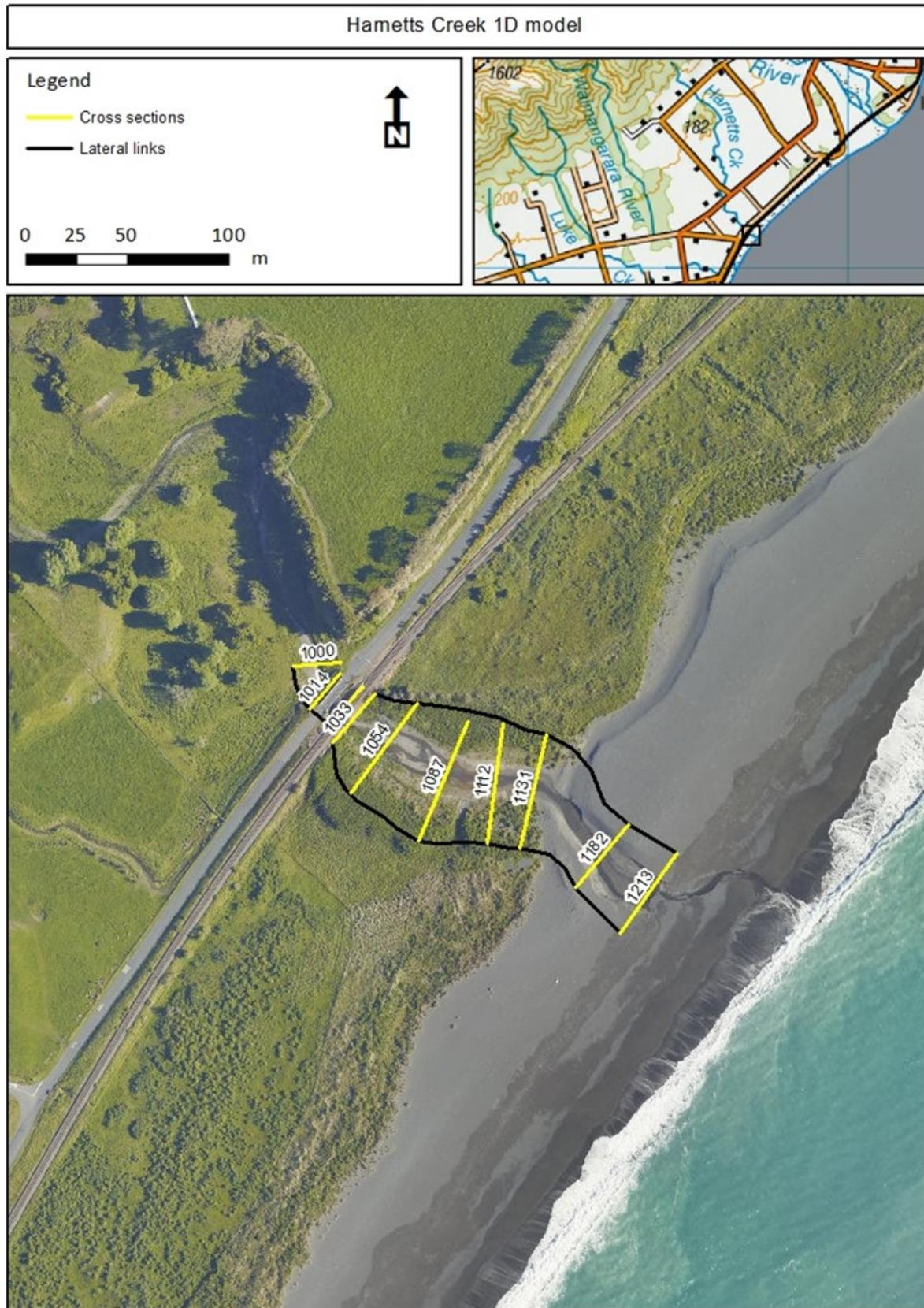
Figure A-6: Harnetts Creek model schematic
