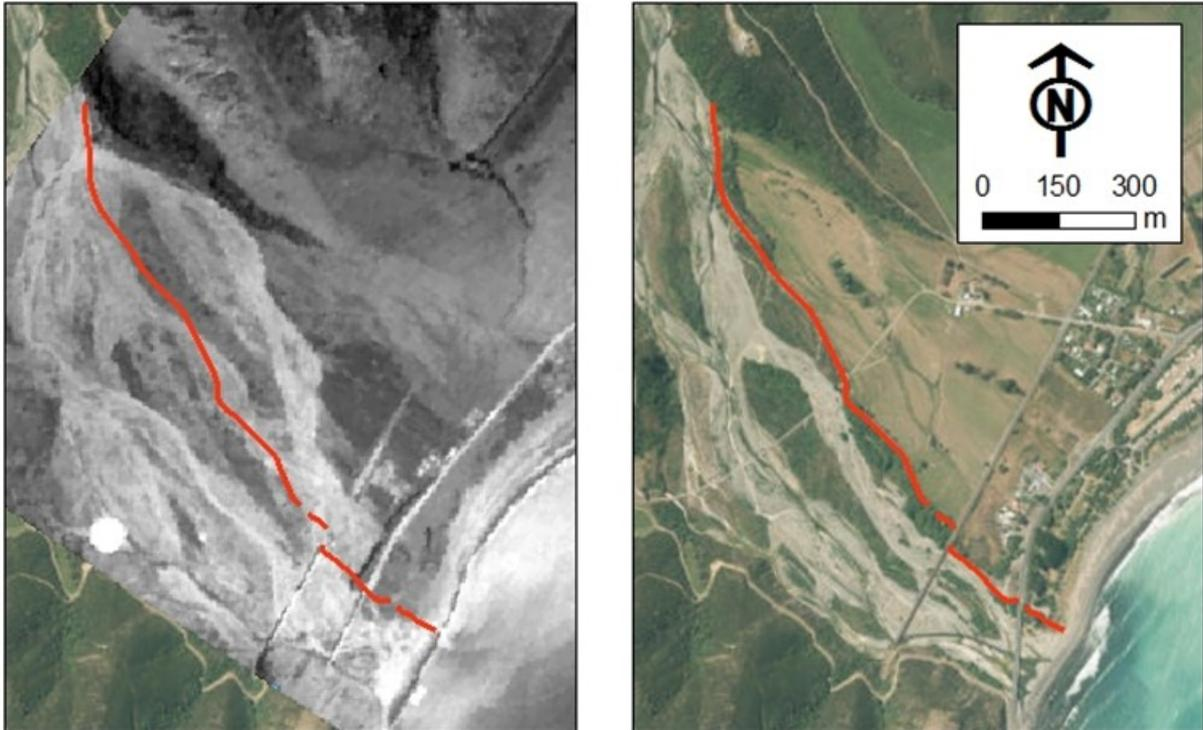
**Figure 2-27: Location of existing flood protection works, along the true left bank of the Kahutara River, superimposed on aerial imagery from 1942 (left) and 2016 (right)**
