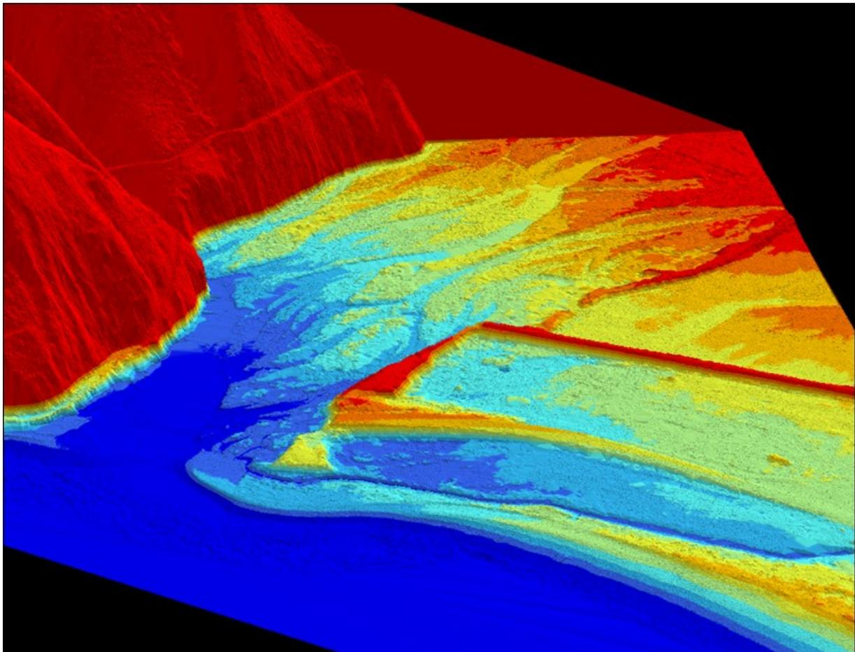
**Figure 3-3: 3D image of the Kahutara River mouth and floodplain LiDAR data (with bridge structures removed and vertical scale exaggerated by a factor of 2)**
