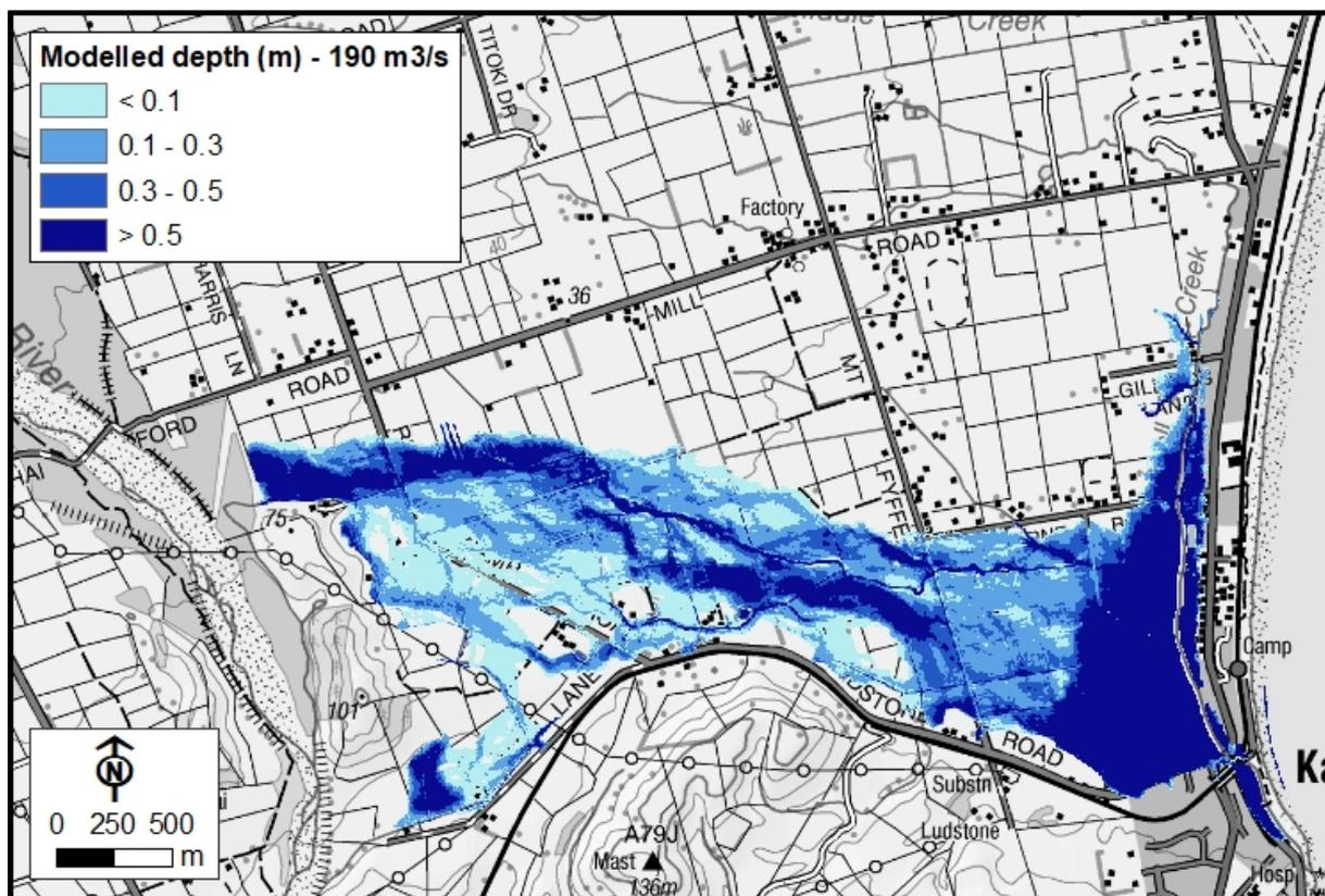
Figure 3-9: Modelled flood depths for the December 1993 flood event (Breakout of 190 m<sup>3</sup>/s)
