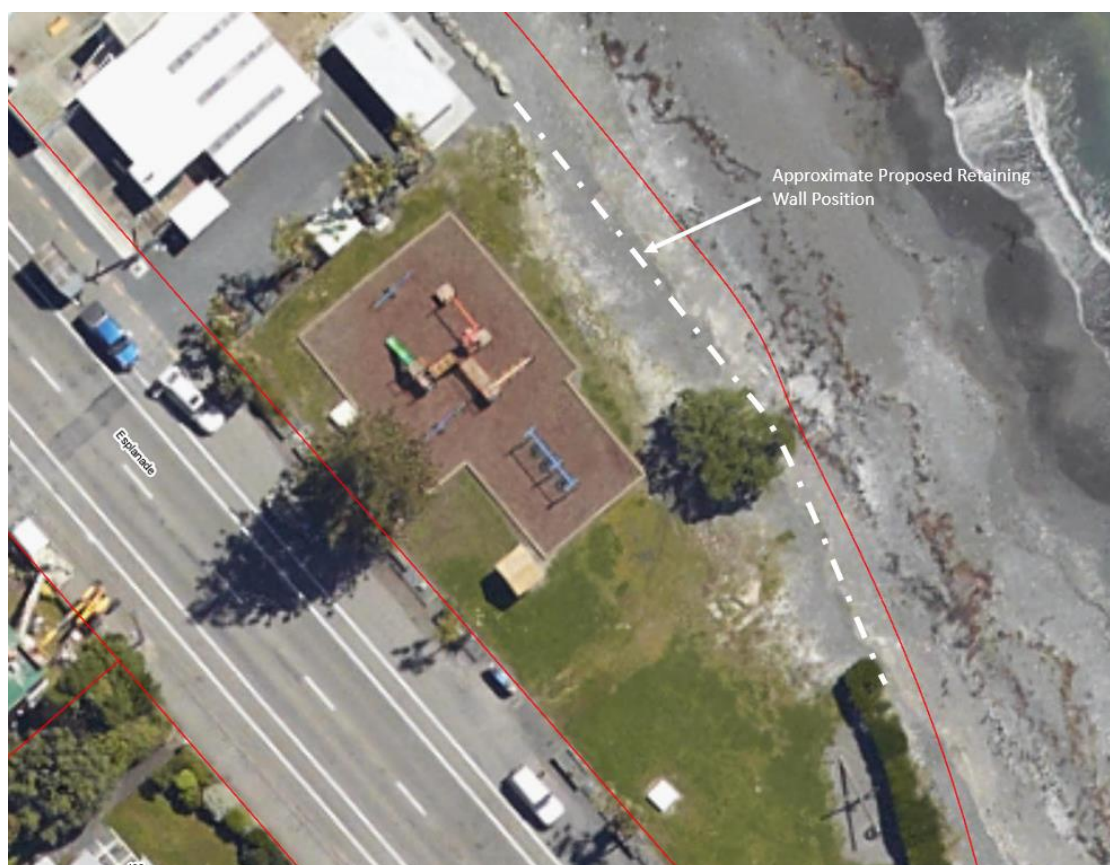
Figure 2 – Proposed Retaining Wall
