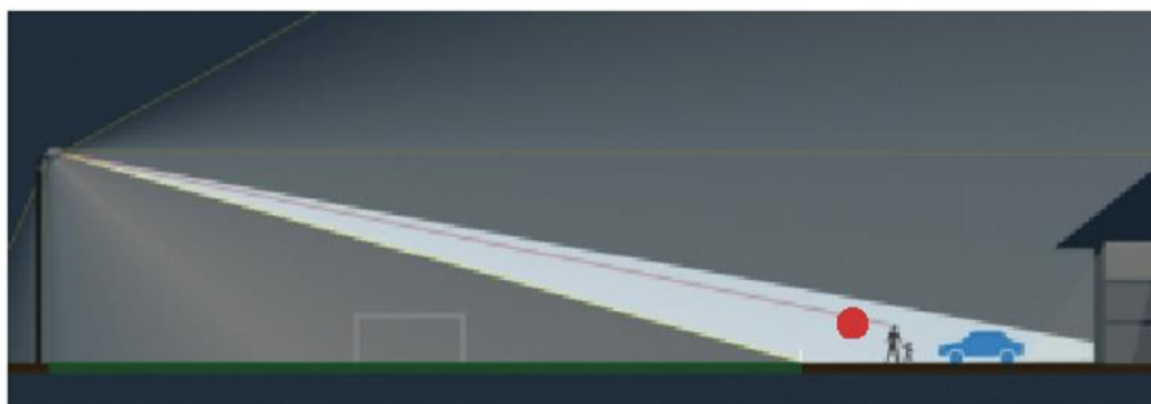
Intensity towards the observer: this concerns the luminous intensity emitted by the luminaire in the direction of the observer.
