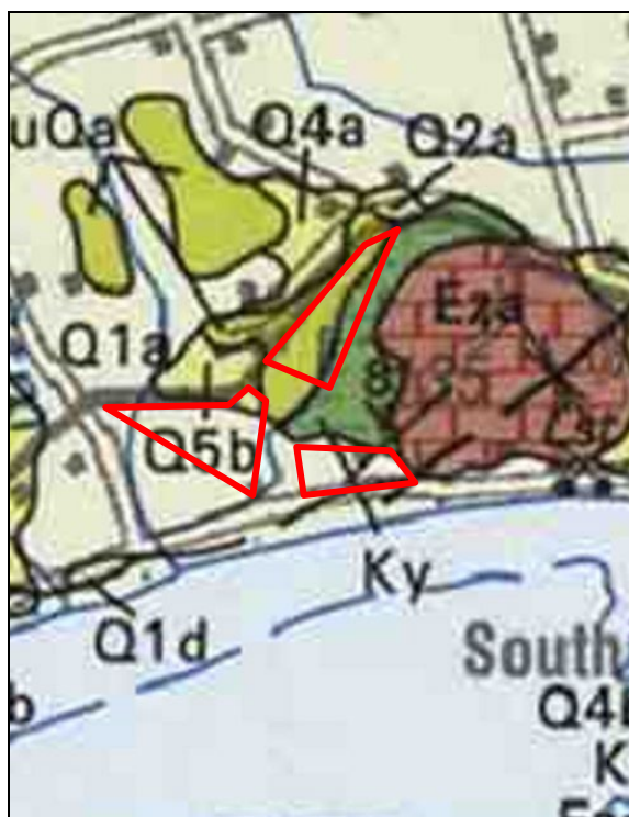
Figure 1: Excerpt from Geological & Nuclear Sciences Geological Map 13, scale 1:250,000, “Kaikoura”. The development areas of the site are roughly outlined in red line.
