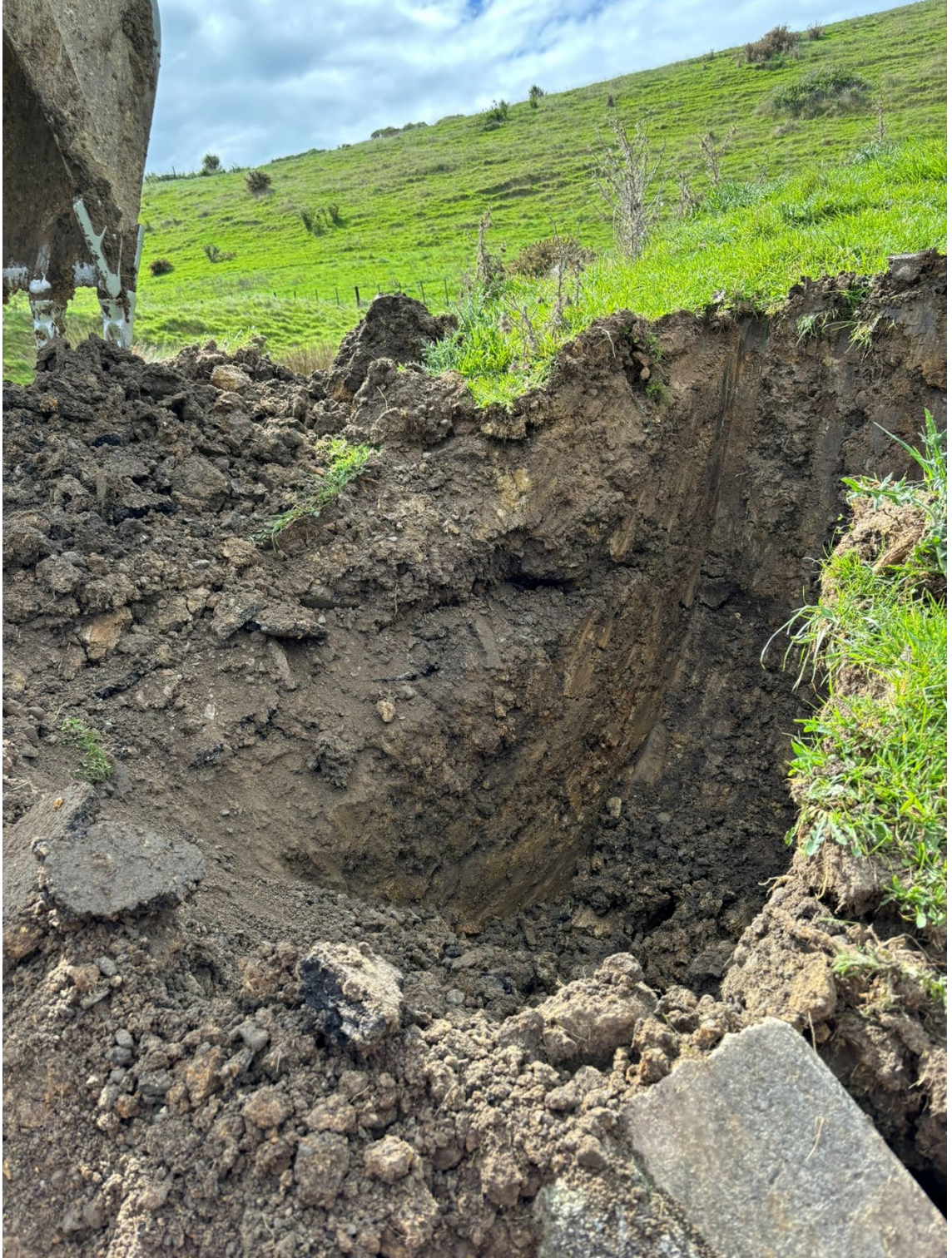
P29: View of test pit put down through one of the overgrown stockpiles (circa 2012). The stockpile generally comprises sandy clayey silts, intermixed with topsoil and trace amounts of concrete and asphalt.
