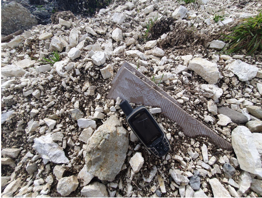
P21: Example of tiles intemixed within stockpiled natural crushed limestone (latest materials to be stockpiled).
