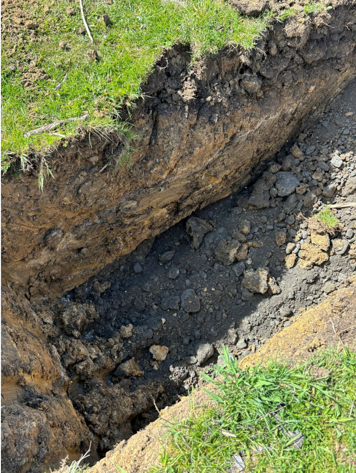
P18: View of test pit put down through clayey silt stockpile (circa 2012). The test pit appears to confirm that the majority of soils in the vegetated stockpiles, are likely to comprise sandy clayey silts, which are in turn underlain by sandy gravels. The sandy gravels in the base of the test pit were not encountered in geotechnical test pits and hand augers put down outside the extent, but in the vicinity of the stockpiles. Thus, these sandy gravels are inferred to be excess imported fill.
