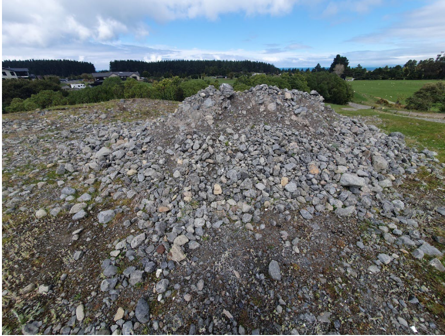
P19: Stockpiled fine to coarse greywacke gravels with some cobbles (circa 2016).
