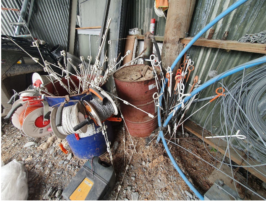
P9: Old 208L drum of diesel engine oil, with an attached pumping apparatus is located in the implement shed. The drum and pump are degraded and do not appear to have been used for a significant amount of time.
