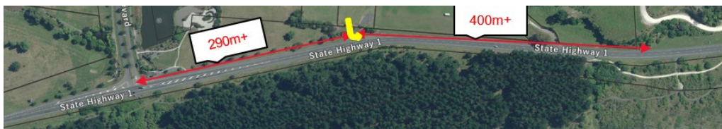
Figure 10: Sight Distance at Proposed Access to SH1
