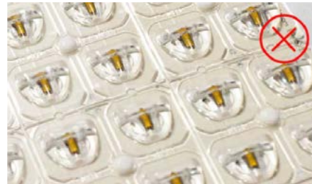
Close-up of a flat array typical of most LED street lights
