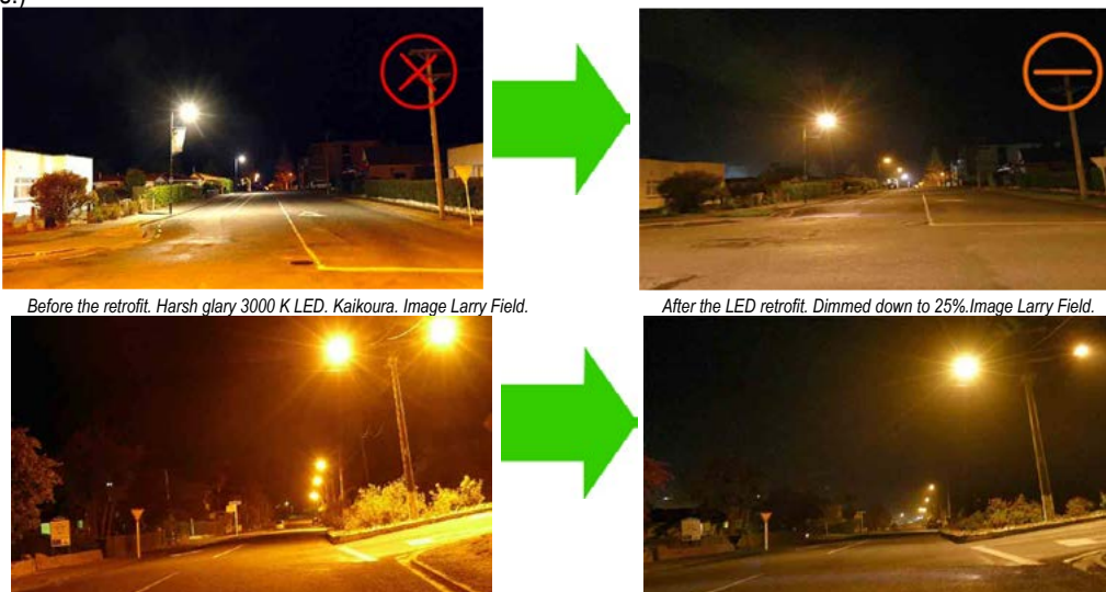
Before the retrofit. Unshielded, HPS lamps Torquay Street, Kaikoura. Image Larry Field.
