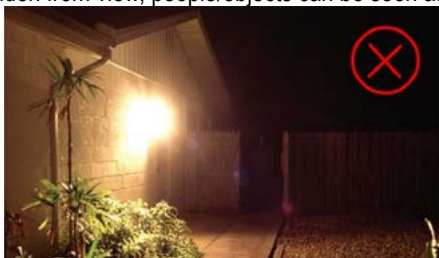
Compromised visibility due to unshielded, glary, high contrast lighting.
