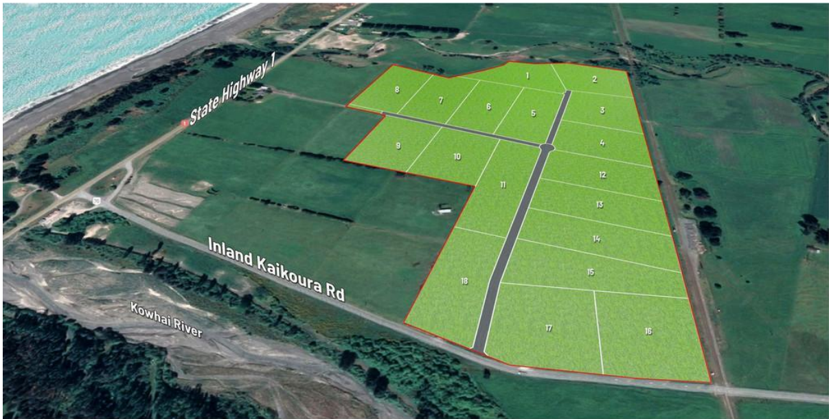
Figure 14. Oblique satellite aerial imagery view of the proposed Kowhai Downs Lifestyle Block subdivision, showing the layout of the 18 2ha lots (overlaid in green) and layout of the sealed access road (overlaid in grey) that will be formed off the Inland Kaikōura Road. Image: https://raywhite.co.nz/marlborough/kaikoura/kaikoura/MET32582/
