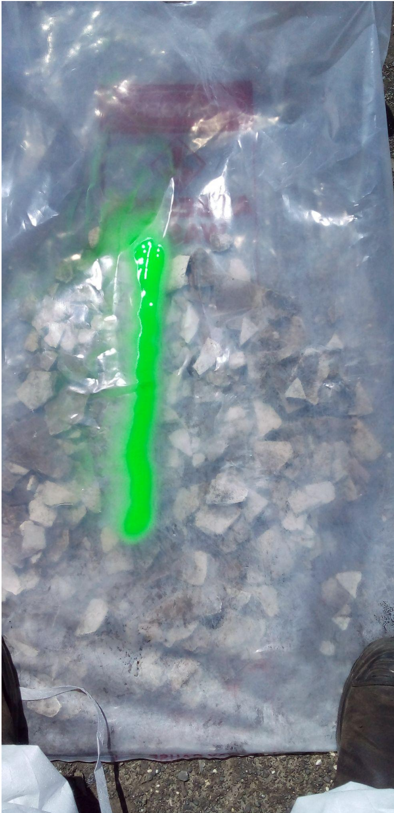
Figure 6. ACM from incinerator area
