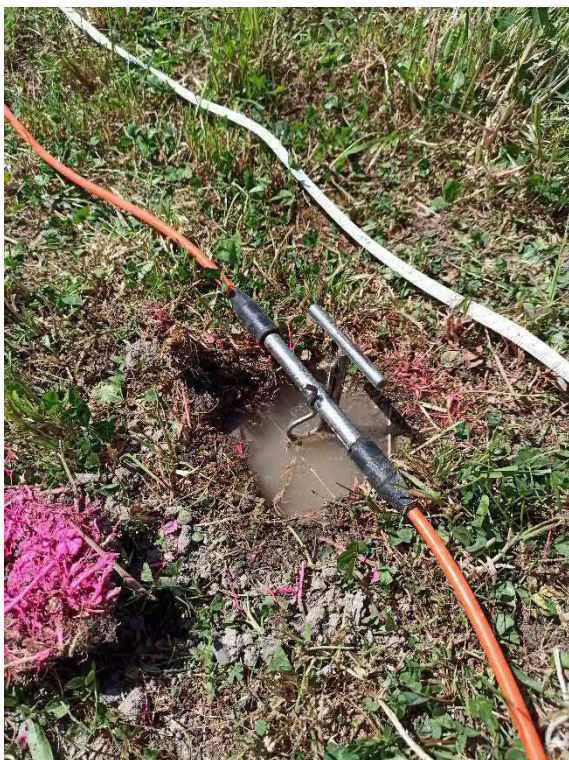
Figure A3: Electrode in small hole with salt water for improved contact resistance
