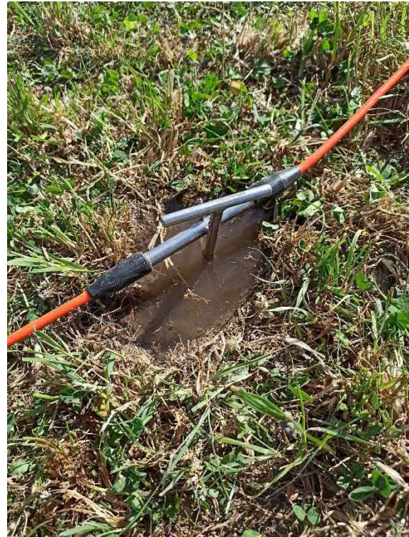
Figure A2: Electrode in small hole with salt water for improved contact resistance
