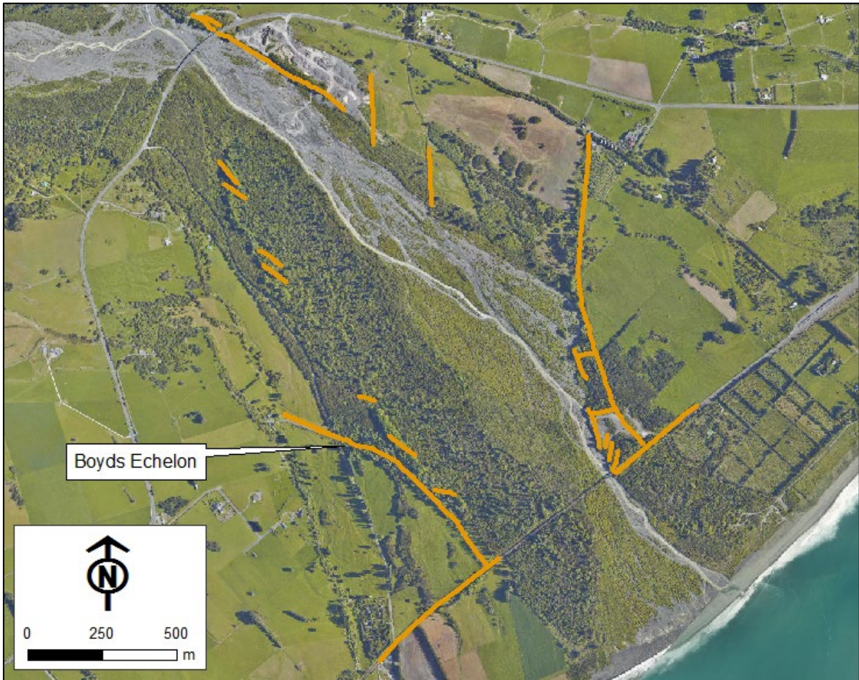
Figure 2-11: Hāpuku River flood protection works (SH1 to the sea)
