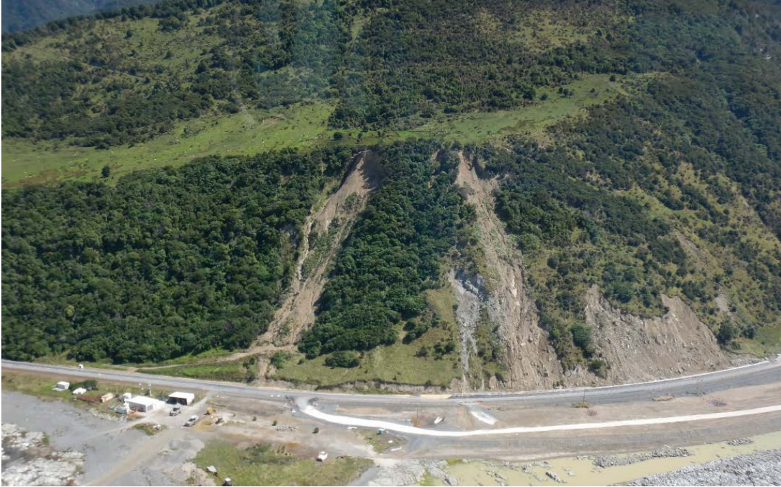
Figure 1.7 Debris avalanches triggered by the 2016 Kaikōura earthquake. Photograph by D. Townsend, GNS Science.
